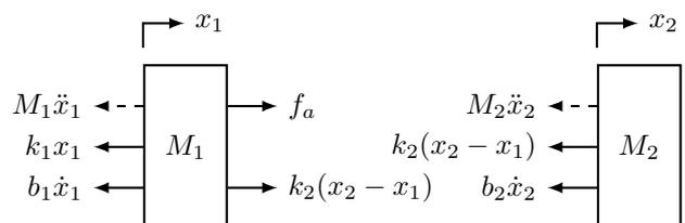
Figure 5: Free body diagram
