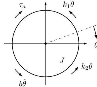
Figure 10: Free body diagram of rotating system.
